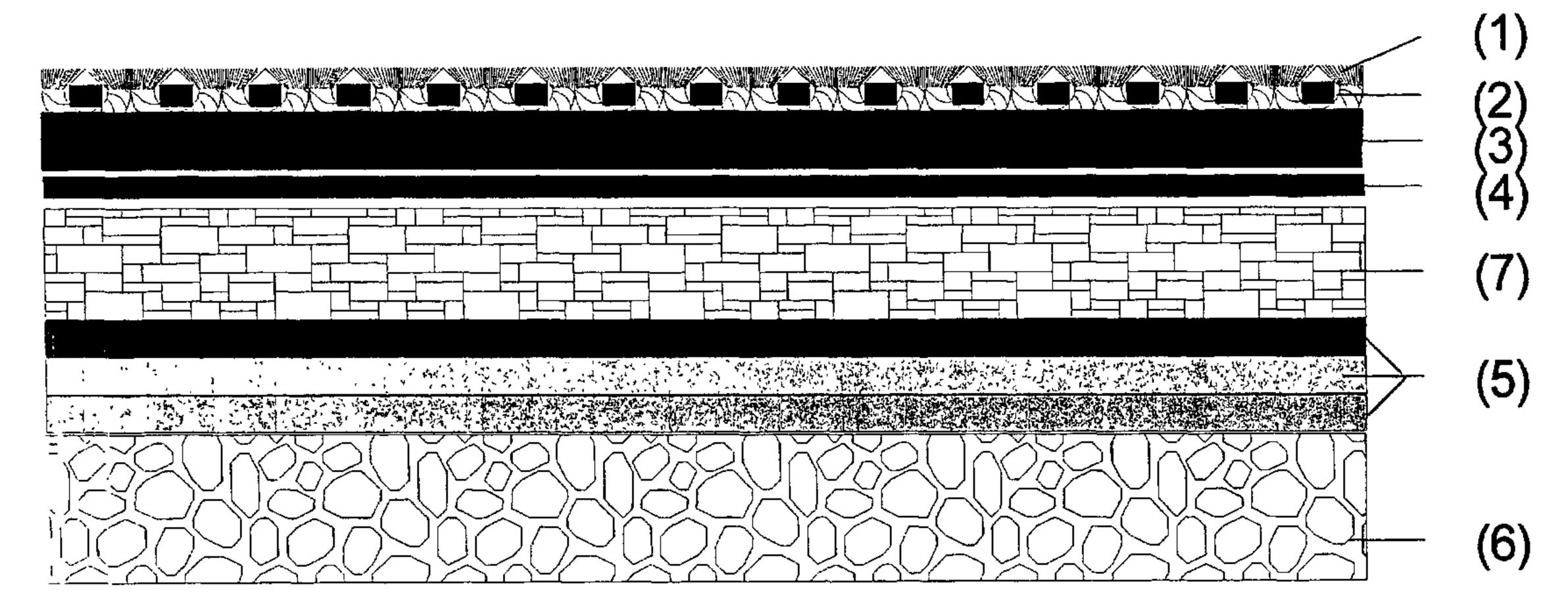
(57) Abstract: A thermoplastic laminate comprising i) a first outer layer comprising an ethylene homo- or co-polymer; ii) a core layer comprising a polyamide; iii) a second outer layer comprising a thermoplastic polyurethane. The thermoplastic laminate is used as an intermediate protective laminate in the manufacture of a polyurethane padded carpet wherein a polyurethane foam layer is formed on the surface of the protective laminate in its turn hot bonded to an upper fibrous layer.
