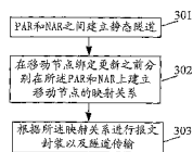
301 ESTABLISH STATIC TUNNEL BETWEEN PAR AND NAR 302 ESTABLISH THE MAPPING RELATION OF MN IN THE PAR AND NAR SEPARATELY BEFORE FINISHING BINDING UPDATE 303 ENCAPSULATE THE MESSAGE AND PERFORM THE TUNNEL TRANSMISSION ACCORDING TO THE MAPPING RELATION
