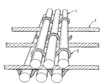
(57) Abstract: A filter element comprising two layers of weft (1) interlaced with warp (2). Additionally laid- in (3) yams are provided in-between the two weft layers. The laid- in yarns (3) are not interlaced with the weft.
