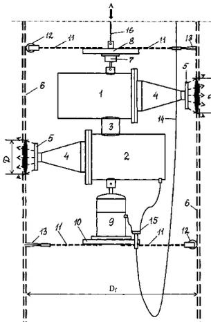
the delivery means causes the acoustic emitter to perform reciprocating movement along the filter axis, thus, providing a subsequent treatment of the entire inner surface of the downhole filter with a directed ultrasonic fluid flow, as well as a regular cleaning of the pre-filter zone of the well without disassembling the water-lifting string and submersible pump.
