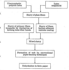
While, generally speaking, any hydrophilic fiber or mixture of such fibers is satisfactory, best results have been obtained with fibers composed of glass and having diameters of less than about 2.5 microns. The fiber diameter should be as small as possible; however, economic and other considerations dictate a preferred range of from 0.2 to 1.5 microns.
