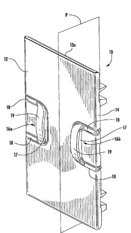
(57) Abstract: A communication cable management system includes a support structure and a door assembly (10). The door assembly includes a door body (12), first (40a) and second (40b) latch mechanisms. The first latch mechanism includes at least two first latch structures 4(5,47). The second latch mechanism includes at least two second latch structure (45,47).
