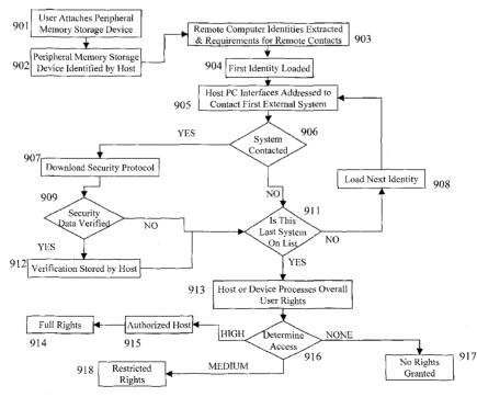
(57) Abstract: A method of secure communication involves determining that a remote system is trusted prior to authorizing secure communication therewith. A removable security device is coupled with a first system. When the first system communicates with a remote system securely, the remote system is evaluated to ensure that it is a trusted remote system prior to secure communication therewith being allowed.
