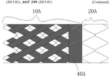
long anchoring area in the main branch vessel so as to ensure that the covered stent has sufficient anchoring force and thus prevent the displacement or endoleak of a distal end of the covered stent, thereby ensuring a good occluding effect.
