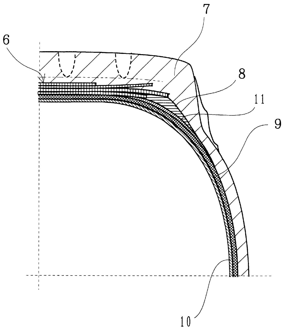
**PNEUMATIC RADIAL TIRE WITH UNDER-BELT PAD AND SPECIFIED INTERMEDIATE RUBBER LAYER RUBBER COMPOUND**
