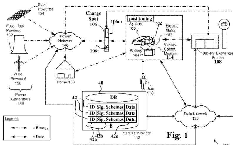
(57) Abstract: Charging management techniques for electrically charging a chargeable device by electrically connecting and disconnecting electric charging power to the chargeable device and selectively performing at least one charging session by a plurality of timely separated charging cycles, depending on power management conditions or instructions.
