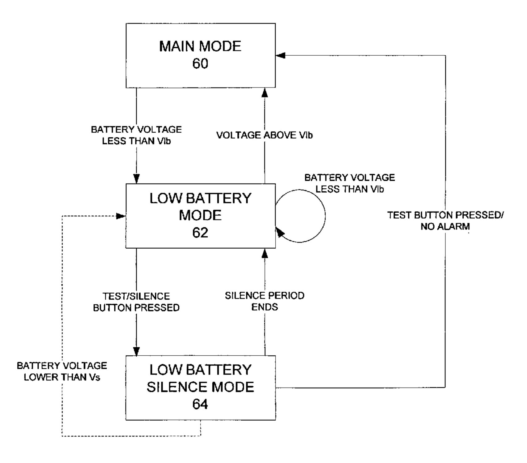
(57) Abstract: A life safety device can include a battery monitoring module configured to measure a voltage level of a battery, an alarm module configured to provide an alarm when the voltage level is less than or equal to a low battery threshold, and a silence module configured to silence the alarm for a random time period.
