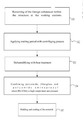
(57) **Abstract**: The present invention relates to a nano-reinforced material with steel and ceramic characteristics by using, in mass ratio, 43 – 50% polyamide, 40 – 42% fiberglass and 10 – 15% polyamide aminopropyl saline (PA-GMA), which functions as a bonder; and the method for production of the said material.
