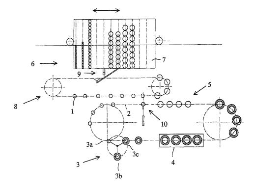
below and an intermediate conveyor (8) and, adapted along the track of the latter conveyor, a mandrel delivery/removal station (9) and a mandrel change station (10), whereby said mandrel delivery/removal station is arranged to operate between said mandrel storage (7) and said intermediate conveyor (8) and said mandrel change station (10) is arranged to operate between said intermediate conveyor (8) and said conveyor track (2).
