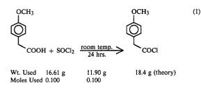
A flask is charged with the carboxylic acid and thionyl chloride and allowed to stand at room temperature with occasional swirling for 24 hours. The endothermic reaction begins immediately and proceeds at a very good rate, generating an orange solution.
