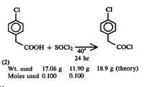
A 50 ml flask is charged with the organic acid and the SOCl<sub>2</sub>. A single boiling chip is added and the flask fitted with air condenser and drying tube. Heating in a  $45^{\circ}$  oil bath is begun. The reaction is cooled after 23 hours.
