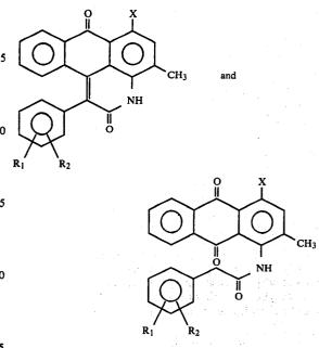
wherein X is Br, I, or Cl, in liquid phase in the presence of a catalytically effective amount of a copper catalyst and at least one mole of inorganic strong base per mole 40 of said anthraquinone at a temperature of from 10° C. to 200° C. for from 0.2 to 24 hours, thereby forming a polymeric red anthrapyridone colorant of the formula
