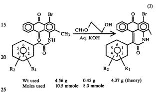
A 100 ml three-necked flask is equipped with watercooled condenser, overhead stirrer, thermowell, and Ar inlet. The flask is charged with the phenylacetyl product of Part (2), and 30 ml methyl cellosolve. The contents are heated to 122° and the KOH in 0.6 ml H<sub>2</sub>O is added dropwise over one minute. The reaction is stirred at 120° for one hour.
