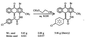
The product of Part (2) and 60 ml of Cellosolve ( $\mathbb{R}$ ) are added to a 250 ml flask. The slurry is heated to 123°. The KOH is dissolved in 1.0 ml H<sub>2</sub>O and added over one minute. The reaction is cooled after heating at 115° for 35 minutes. The mixture is allowed to cool slowly to room temperature and then cooled to 5° C. A solid <sup>45</sup> precipitate is isolated and washed to afford 3.32 g of glittering, brownish/golden crystals.
