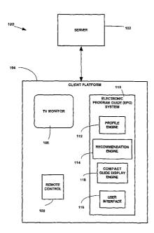
(57) Abstract: In a content distribution system (100), in which broadcast content is distributed and provided by a server (102) to a television viewer using a client platform (104), a method and apparatus for providing a compact guide display of a plurality of television show or program recommendations, optionally with descriptions, which are available and selectable for viewing by a viewer without interrupting the presently-viewed content.
