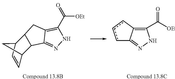
[0333] Compound 13.8B was prepared from the corresponding ketone using a similar method as described herein for the preparation of pyrazole esters (see Example 13.1 and 13.2). A solution of Compound 13.8B (2.0 g, 8.19 mmol) in phenyl ether (25 mL) was heated at reflux (250~260° C.) under nitrogen for 2 hours.
