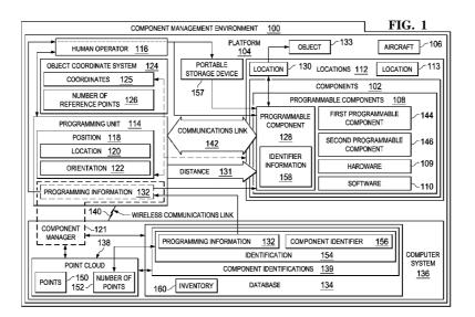
(57) Abstract: A method and apparatus for managing a programmable component may be present. A location on an object may be identified using a programming unit based on a position of the programming unit with respect to the object. Programming informa tion for the programmable component may be identified based on the location on the object. The programmable component may be programmed using the programming information for the programmable component.
