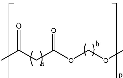
wherein each of a and b may range from 1 to 12, from 2 to 12, or from 4 to 12, and further wherein p may range from 10 to 100, from 20 to 80, or from 30 to 60. In embodiments, the crystalline polyester is poly(1,6-hexylene-1,12-dodecanoate), which may be generated by the reaction of dodecanedioic acid and 1,6-hexanediol.
