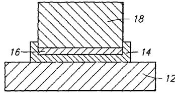
(57) Abstract: The invention includes methods of reducing grain sizes of materials, and methods of forming sputtering targets. The invention includes a method for producing a sputtering target material in which a metallic material is subjected to plastic working at a processing percentage of at least 5 % and a processing rate of at least 100 %/second. In particular applications the metallic material comprises one or more of aluminum, copper and titanium.
