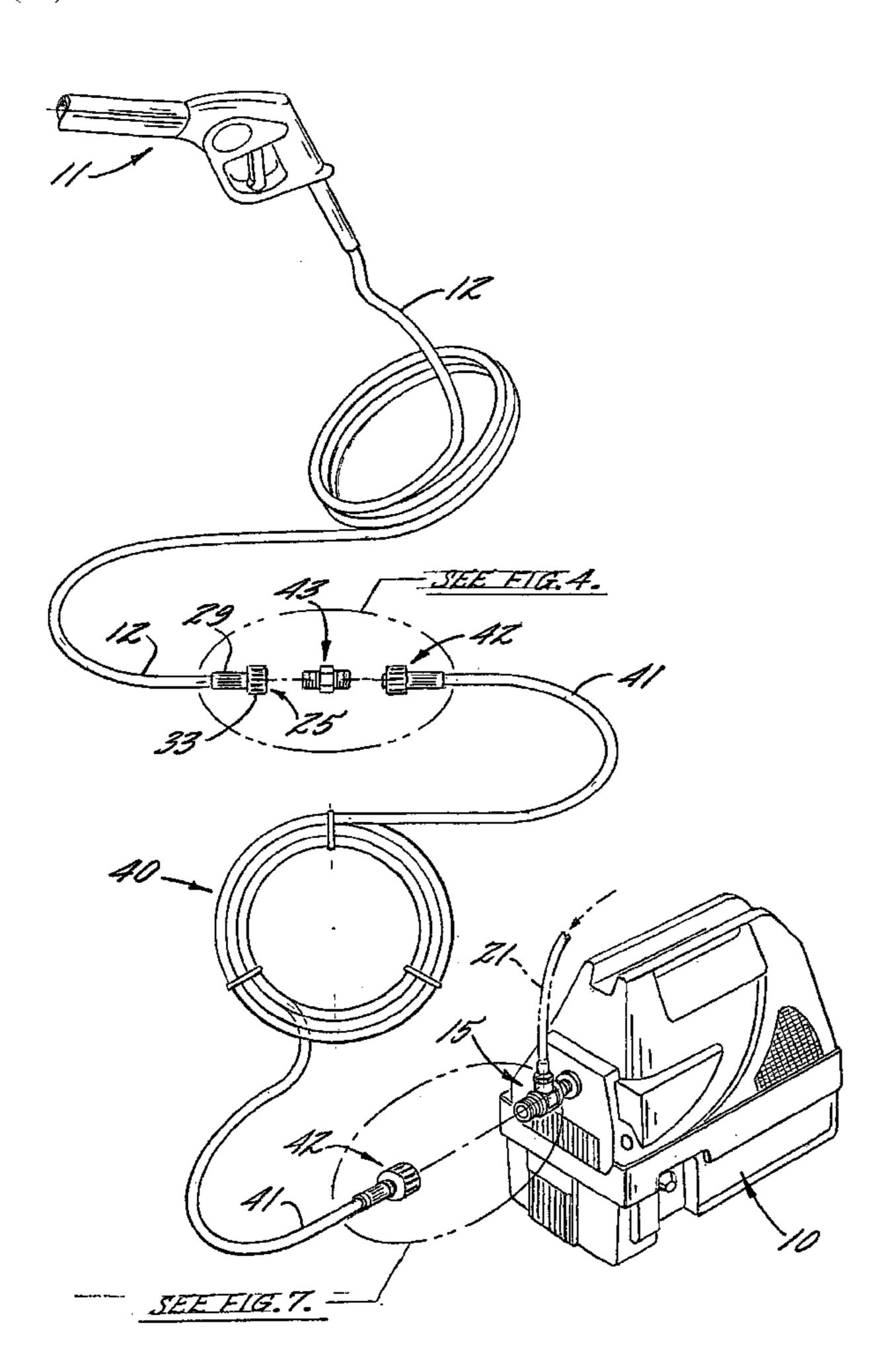
(57) Abstract: A universal pressure washer extension/replacement hose adapted for use with pressure washers which have different diameter liquid discharge outlets. The extension hose has identical connecting fittings at its opposite ends, one of which can be coupled in sealed relation to a pressure washer outlet of either of two known sizes and the other of which is connectable to a spray gun hose through a universal adaptor having connecting chambers of said two known sizes.
