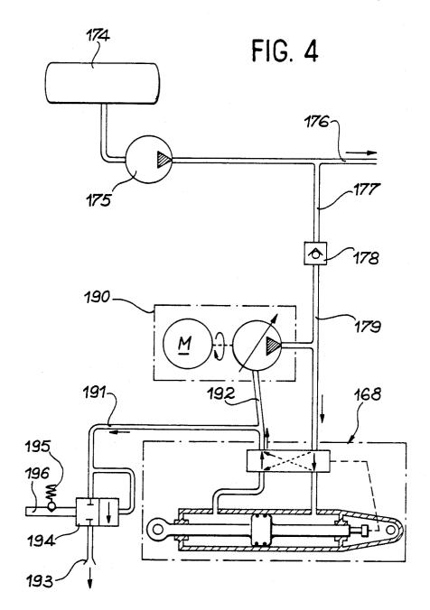
LOST-FLUID HYDRAULIC ACTUATION SYSTEM
