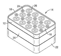
needed energy burst to support the scanning/reading operation. Each electrode measures the equivalent sub-epidermal capacitance corresponding and representing the moisture content.
