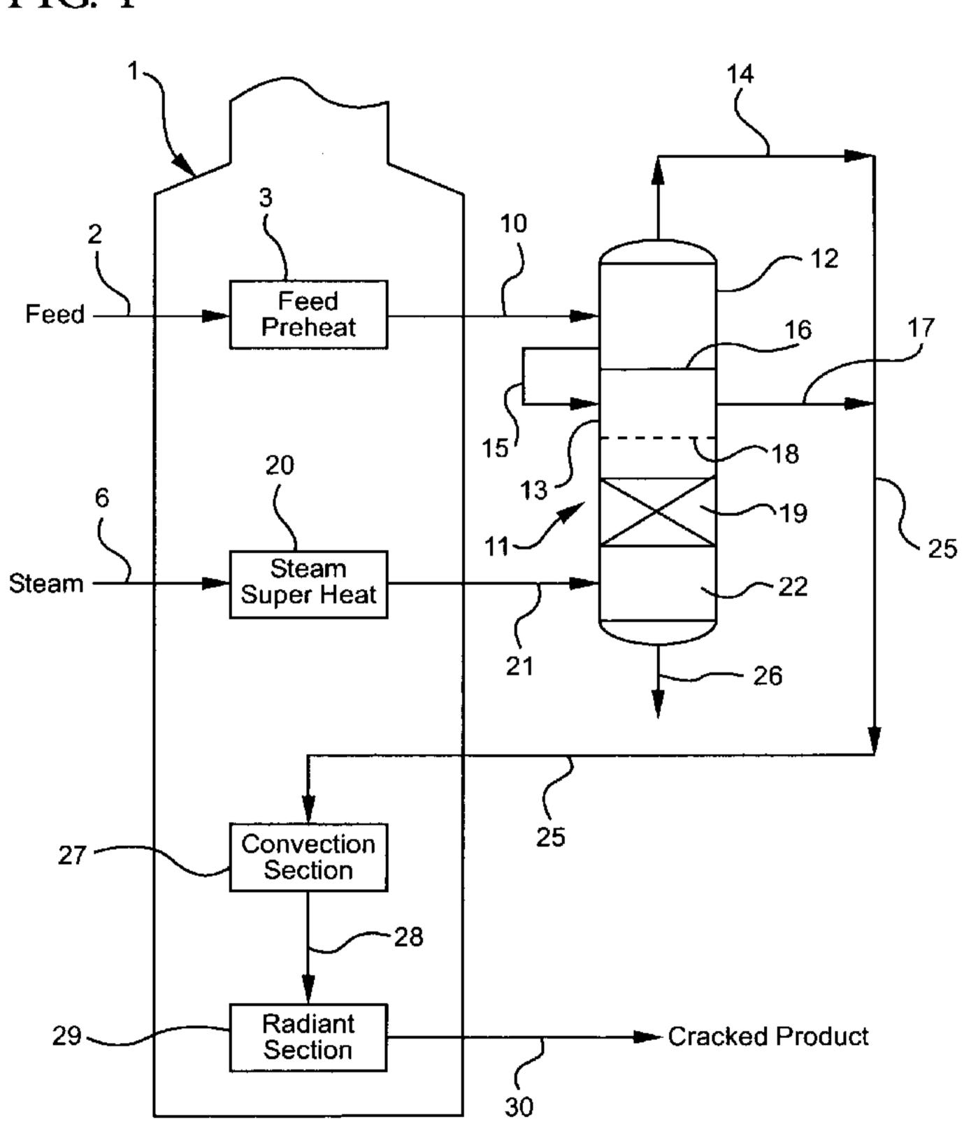
(57) Abstract: A method for thermally cracking an organic acid containing hydrocarbonaceous feed wherein the feed is first processed in a vaporization step, followed by thermal cracking.
