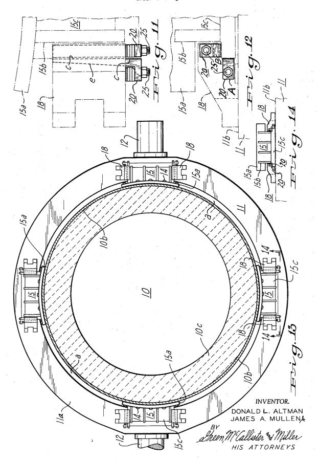
The invention pertains to an improved mounting and support for a molten material handling or processing vessel such as a furnace vessel, and particularly to a so-called stabilizing type of trunnion mounting which makes use of gibs or keepers having cooperating wedging elements, that are carried by the trunnion ring, and that cooperate with associated mounting brackets that are secured to project from the vessel.
