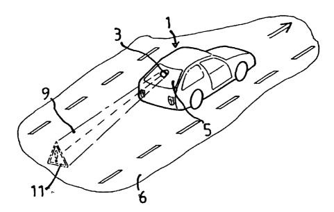
(57) Abstract: The invention concerns a visual signalling device adaptable to a running vehicle (1), comprising a rear emitter (3) for emitting a laser beam (9) towards the rear of the vehicle (1). The invention is characterised in that the rear emitter (3) comprises means generating designs for projection, by the laser beam, of a signalling design (11) at the rear of the vehicle. The invention is applicable to equipment for motor vehicle, bus, boat.
