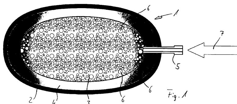
(57) Abstract: The invention relates to a cushion having damping properties for bicycle pants. The cushion comprises an outer shell (2) and a core (3) and at least one layer (4) arranged between the outer shell (2) and the core (3). The core (3) and the layers (4) are formed by at least one filler material having different degrees of firmness. The damping properties of the core (3) and/or of the layers (4) can be changed by means of inflation.
