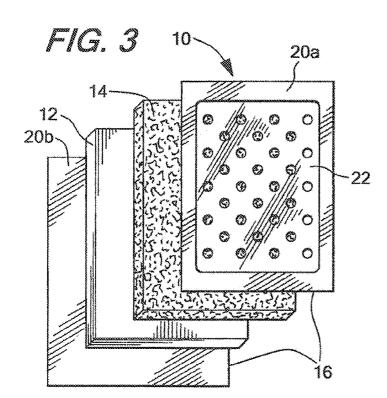
(57) Abstract: An oxygen based heater including a heater substrate and a pad impregnated with an electrolyte solution disposed adjacent to the heater substrate which transfers electrolyte to the heater substrate. Methods of manufacturing same in an oxygen containing environment in which electrolyte is impregnated onto pad which is adjacent heater substrate.
