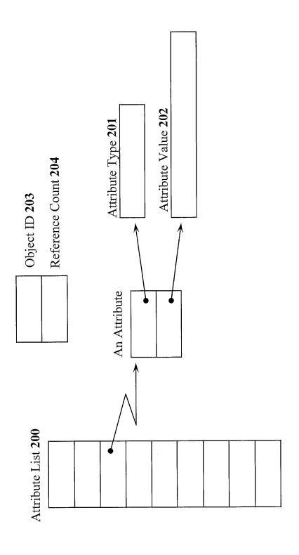
Fig. 2: Structure of a Viewing Object
