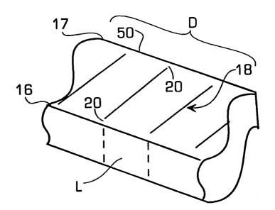
membrane stretching. Once properly scribed to the desired dimension, these dies can be further processed including utilizing the scribes to produce square ends to produce precise reflective laser cavities.
