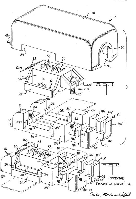
ELECTRICAL CONNECTOR ASSEMBLY FOR INSULATED TAPE CABLE
