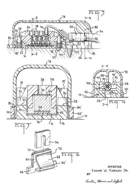
ELECTRICAL CONNECTOR ASSEMBLY FOR INSULATED TAPE CABLE
