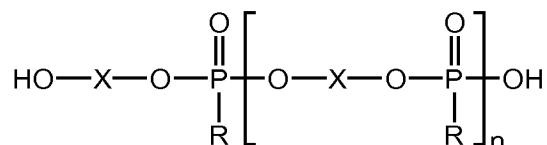
wherein R is a C<sub>1</sub> to C<sub>20</sub> alkyl or, optionally substituted, aryl group, X is an aromatic, cycloalkyl, or aliphatic group, and n is an integer of from 1 to about 10
