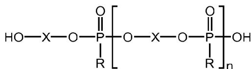
wherein R is a C<sub>1</sub> to C<sub>20</sub> alkyl or, optionally substituted, aryl group, X is an aromatic, cycloalkyl, or aliphatic group, and n is an integer of from 1 to about 10. In certain embodiments, the one or more oligomeric phosphonates have a phosphorous content of about 2% to about 12% by weight. In particular embodiments, the compositions may include about 5 wt. % to about 60 wt. % of the one or more oligomeric phosphonates.
