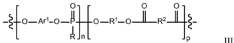
and combinations thereof, where Ar, Ar<sup>1</sup>, and Ar<sup>2</sup> are each, independently, an aromatic group and -O-Ar-O- may be derived from a dihydroxy compound having one or more, optionally substituted
