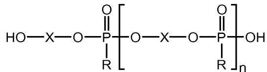
wherein R is a C<sub>1</sub> to C<sub>20</sub> alkyl or, optionally substituted, aryl group, X is an aromatic, cycloalkyl, or aliphatic group, and n is an integer of from 1 to about 10
