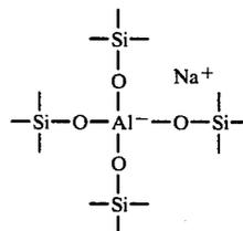
After treatment with a complexing agent such as ethylene-diaminetetraacetic acid (H<sub>4</sub>EDTA) in which a stoichiometric reaction occurs whereby framework aluminum atoms along with an associated cation such as sodium is removed as NaAlEDTA, it is postulated that the tetrahedral aluminum is replaced by four protons which form a hydroxyl "nest", as follows:
