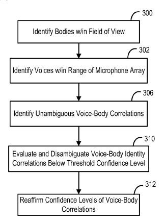
(57) Abstract: A system and method are disclosed for tracking image and audio data over time to automatically identify a person based on a correlation of their voice with their body in a multi-user game or multimedia setting.
