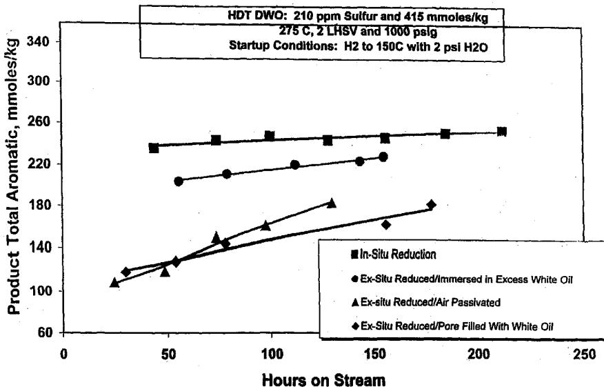
(57) Abstract: A method of ex-situ activation and dry passivation of supported noble metal catalysts including the steps of reducing in the presence of hydrogen and dry passivation by cooling in an inert atmosphere and exposing to air or by filling the pores of the catalyst with a low sulfur oil before exposing to air.
