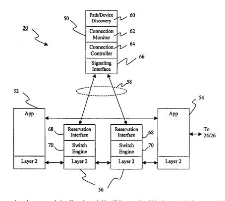
packets to an enterprise control point for processing via a reserved signaling channel, identifying a path within the network that can satisfy the requested QOS/COS and reserving the requested resources all along the path from beginning to end.
