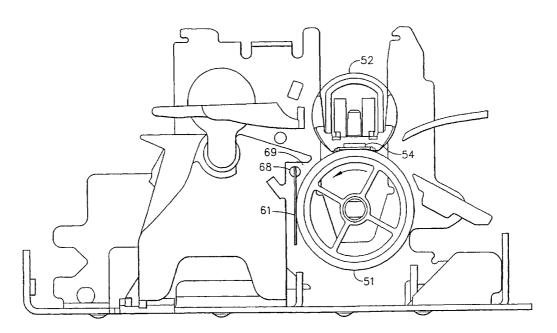
(57) Abstract: An image-fixing device for use in an electrophotographic process which includes a wiping member (61), (62), (64), (67) in contact with the back-up roller (51) of the fusing portion of the device. This wiping member has a high surface energy which eliminates moisture condensation on the back-up roller (51). This acts to eliminate stalls and paper jams without requiring major reformulation of the composition of the fuser belt or back-up roll or the structure of the printer.
