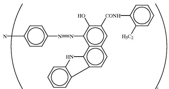
Then a charge carrier transport layer, which consisted of a mixture of the charge carrier transport material having formula (c) and a polycarbonate resin (Trade name of PANLITE K-1300, manufactured by Teijin ltd.) in a ratio of 1:1 by weight was formed thereon such that the thickness thereof was 20  $\mu$ m.
