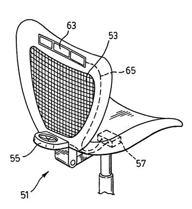
(57) Abstract: A chair (1), bed, lounge or other similar type structure has electrical functions or features and also has an energy converter (21, 9, 59) which produces electrical power from conditions to which the structure is exposed on a regular basis to power the functions or features.
