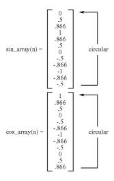
[0033] The proper indexing of the sine and cosine array values in the above look-up table provide for computing of the proper four quadrant phase (0-360 degrees) result that is computed based on the final in-phase and quadrature phase results. As appreciated, the example look up tables are directed to the disclosed example including 12 samples. The example look up tables could be modified to match the number of desired samples.
