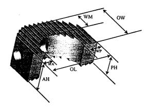
AH- anterior height PH-posterior height WA-anterior width WP-posterior width OL-overall length OW-overall width WM-medial width
