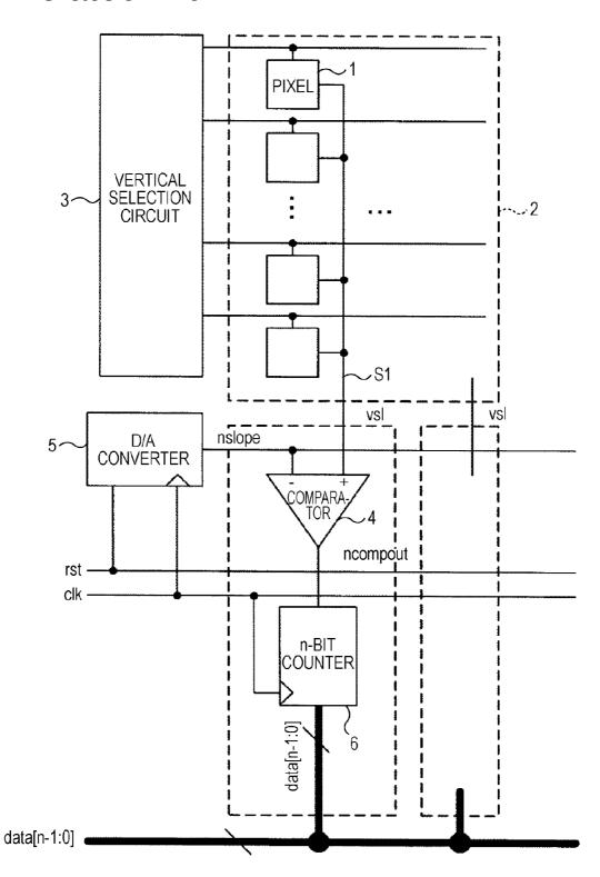
STOP COUNTDOWN WHEN OUTPUT OF COMPARATOR GOES FROM L TO H Related Art uslope – ncompout -픙 ß <u>\s</u>
