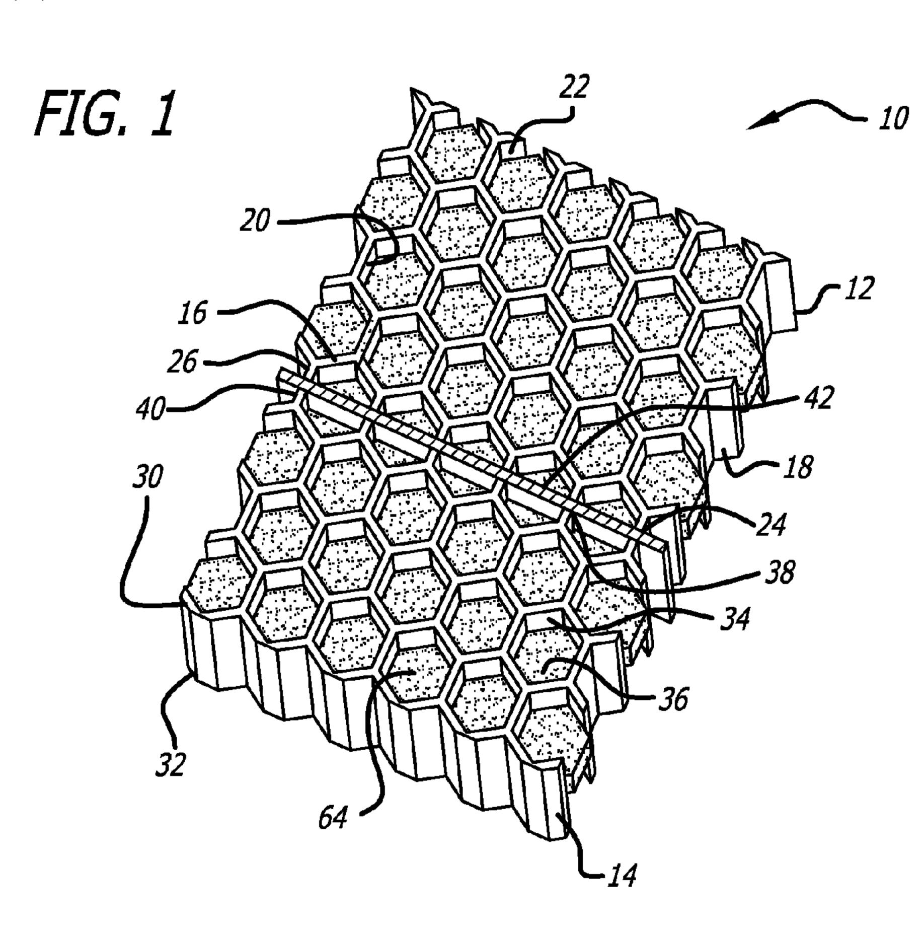
(57) Abstract: Honeycomb sections are bonded together with seams made up of an adhesive that is carried by a honeycomb seam support or a linked-segment seam support. The seams are particularly useful for splicing together curved honeycomb sections that contain acoustic septum. The curved acoustic honeycomb sections are spliced or seamed together to form engine nacelles and other acoustic dampening structures.
