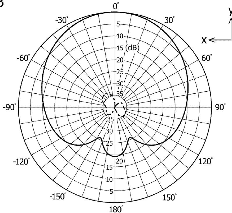
[HORIZONTALLY POLARIZED WAVE IN THE TRANSMITTING BAND]
