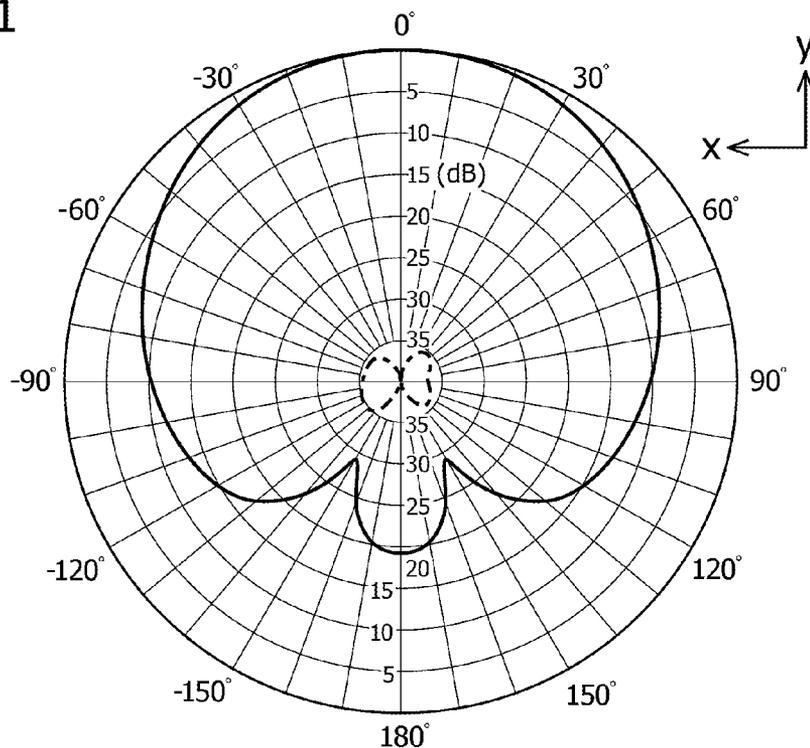
[HORIZONTALLY POLARIZED WAVE IN THE RECEIVING BAND]
