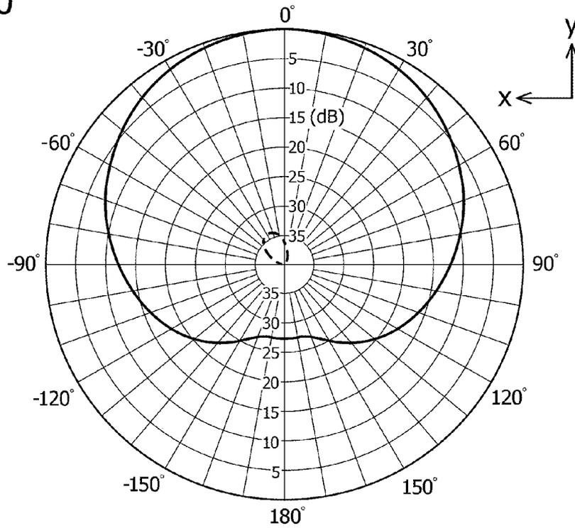
[VERTICALLY POLARIZED WAVE IN THE RECEIVING BAND]
