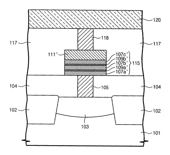
PHASE CHANGE STORAGE CELLS FOR MEMORY DEVICES, MEMORY DEVICES HAVING PHASE CHANGE STORAGE CELLS AND METHODS OF FORMING THE SAME
