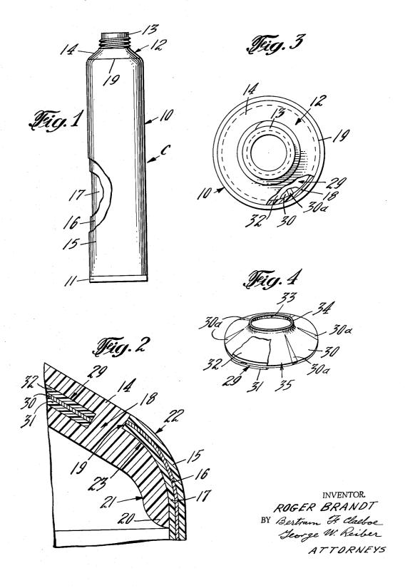
METHOD OF MAKING A COLLAPSIBLE CONTAINER STRUCTURE
