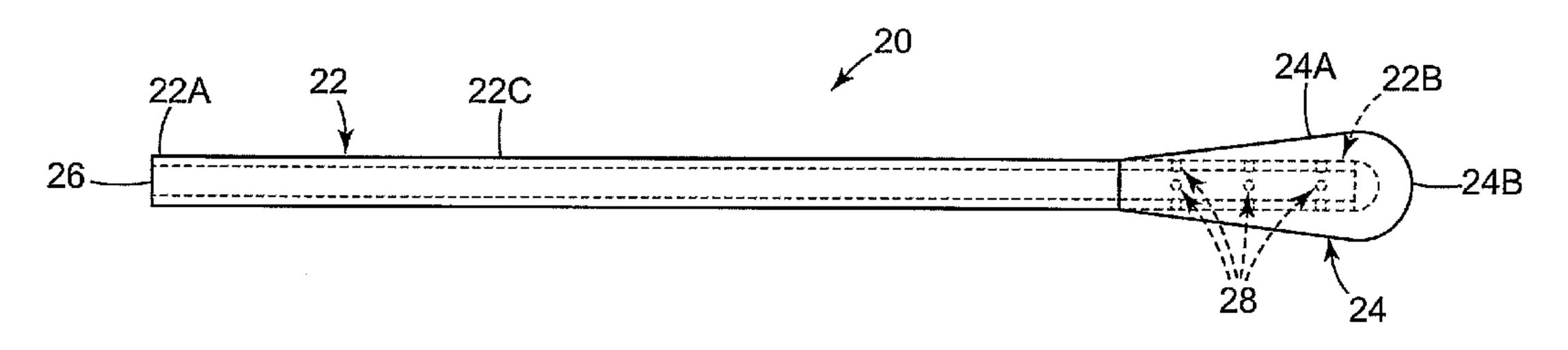
(57) Abstract: A sample acquisition device includes a hollow shaft and a porous medium. The hollow shaft includes a proximal end, a distal end, and a sidewall extending between the proximal end and the distal end. The sidewall of the hollow shaft includes a plurality of openings adjacent the distal end of the hollow shaft. The porous medium is attached to the distal end of the hollow shaft and at least a part of the porous medium is positioned over the plurality of openings.
