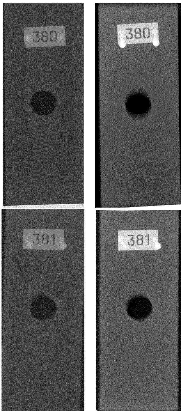
Figure 2 : X-ray images of tralopyril impregnated wood samples after 1 and 2 years
