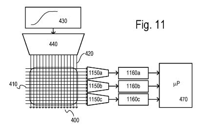
(57) Abstract: Disclosed is a touch sensitive display apparatus comprising a sensor comprising an input array of electrodes and, capacitively coupled thereto, an output array of electrodes. The apparatus also comprises a plurality of reception circuits (for example three), each reception circuit being operable to simultaneously receive a signal from a different electrode of said output array of electrodes. The reception circuits each comprise an analogue to digital converter.
