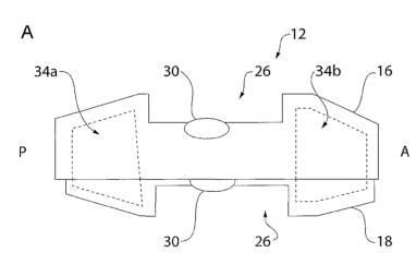
(57) Abstract: An intervertebral implant, or disc prosthesis, comprises a pair of cooperating elements being provided in a generally "X" shaped structure. The elements are comprised of cooperating shells that are maintained separated by a resilient material provided therebetween. The elements allow for rotational and translational movement when implanted.
