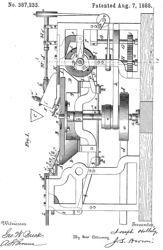
MACHINE FOR BEVELING THE EDGES OF GLASS PLATES.
