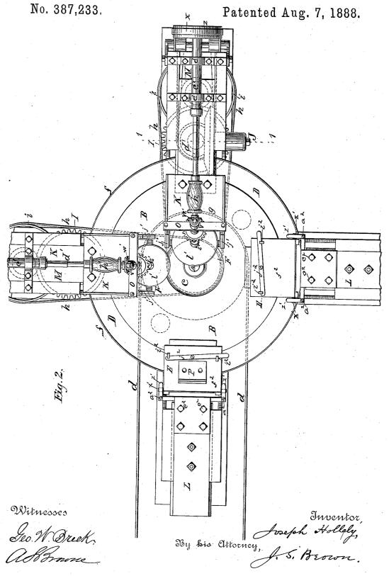
MACHINE FOR BEVELING THE EDGES OF GLASS PLATES.
